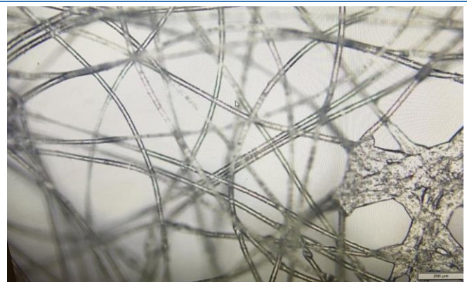
Fig. 3. Optical image of the surgical mask without the MAYA Sticker (scale bar: 200 μm).
